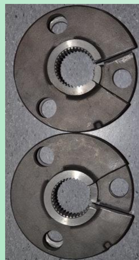
Sectioned planetary gears
